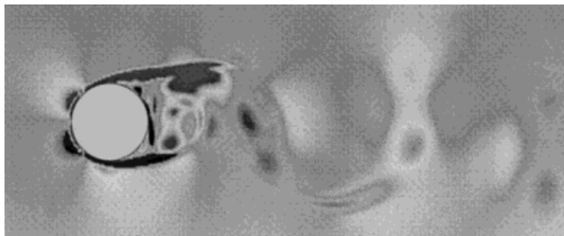
Figure 20. Vorticity field. Re = 400 - \tilde{\Omega} = [0, 20] \times [0, 5] —non-uniform mesh 512 \times 128 .
